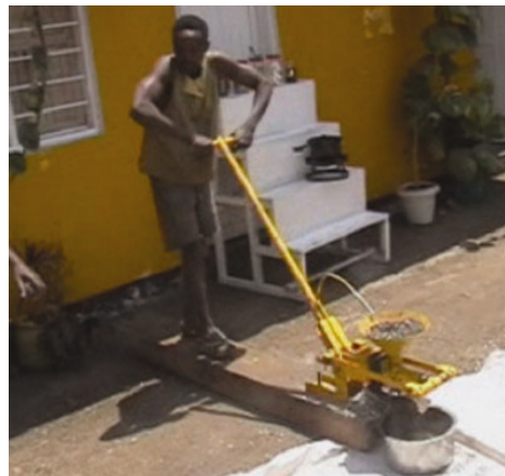
Figure 9: Jatropha oil extraction using a Bielenberg ram press. Source: (FACT 2006).
