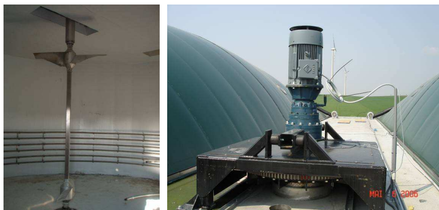
Figure 7.23 Hanging paddle stirrers (left) and its stirring engine (right) (AGRINZ 2006)
