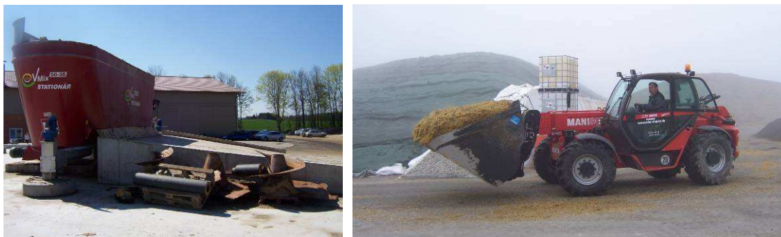
Figure 7.10 Feed-in container system for dry feedstock -maize silage and solid poultry manure- (left) and loader with maize silage (right) (RUTZ 2008)
