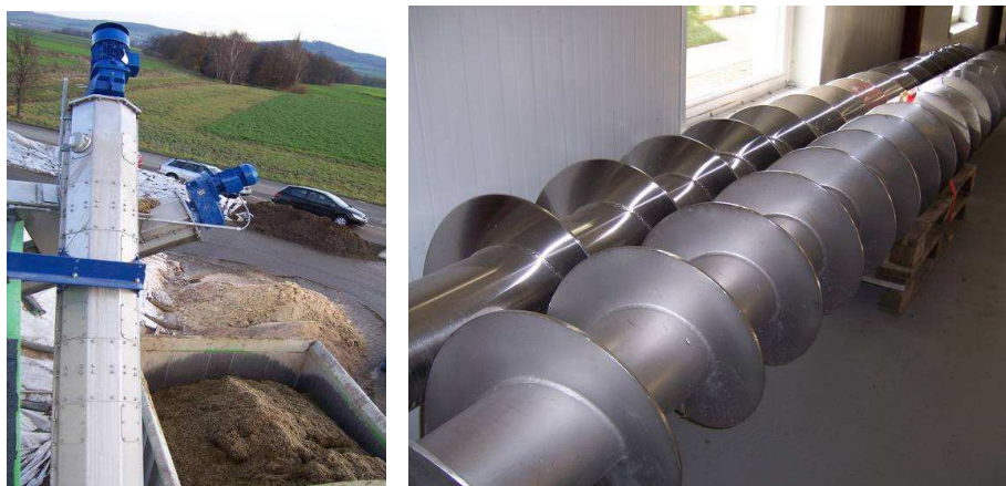
Figure 7.12 Screw pipe transporting system ( left ) and conveyor screws, ready for installation ( right ) (RUTZ 2007)
