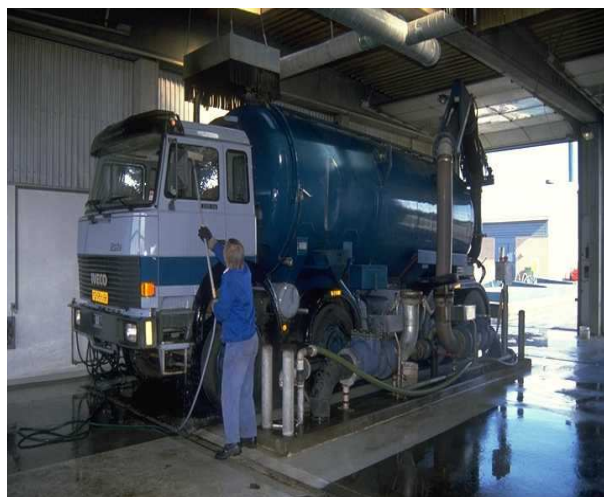
Figure 9.1 Example of standard cleaning procedure from Ribe biogas plant in Denmark
