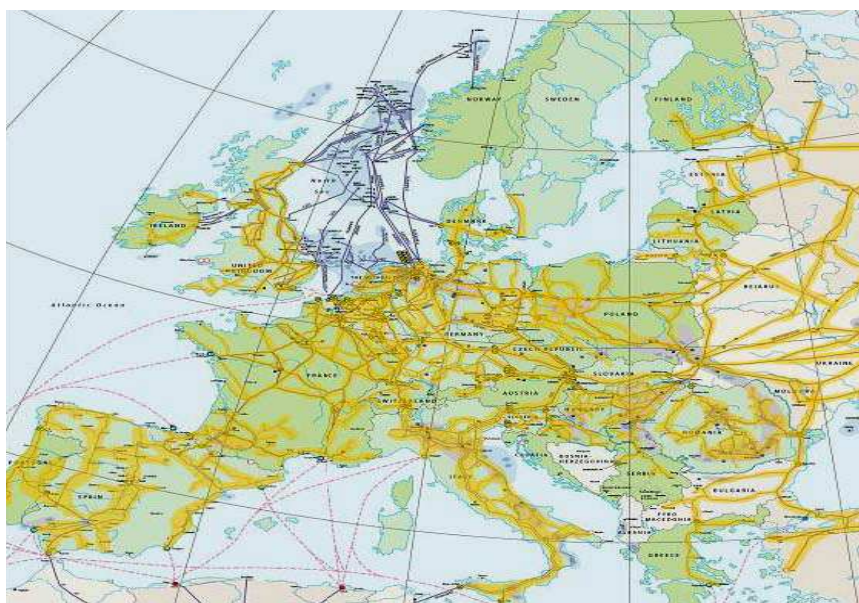
Figure 2.1 European natural gas grid and potential corridors (yellow) suitable for biogas production and biomethane injection (THRÁN et al. 2007)
