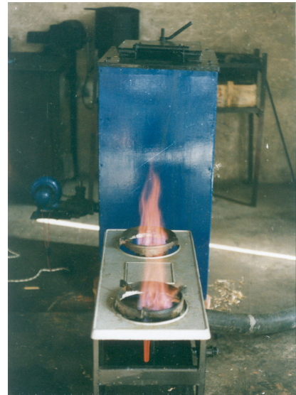
Fig. 4: cooking stove using medium heating value gas (bio-syn-gas).
