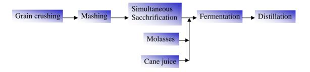
Fig. 10.3 Simplified Process Flow sheet for Production of Ethanol
