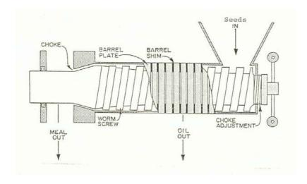
Fig.10.1 Principle of Oil Expeller Operation
