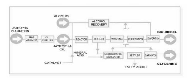
Fig. 10.2 Simplified Process Flow sheet for Production of Biodiesel
